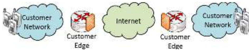
Figure 10: Policy-based communication via CES firewall at network edges
